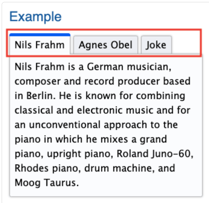
Figure 8.14. Element with the tabList role (Source: W3C 386 )
